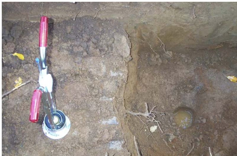
Figure 7 Turf-Tec Infiltrometer at shallow bench and percolation hole at deeper bench
