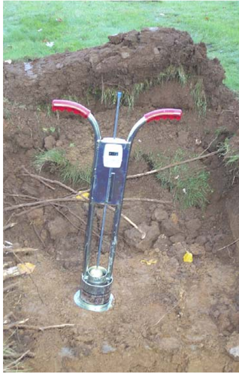
Figure 6 Turf-Tec Infiltrometer – example of double ring infiltrrometer
