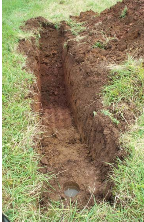
Figure 1 Deep Hole Test Indicating Multiple Horizons.
